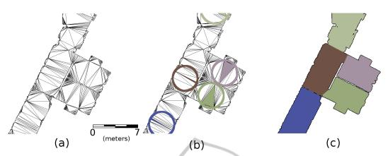
Figure 3: Example room seed partitioning: (a) interior triangulation; (b) the room seed triangles, and their corresponding circumcircles; (c) room labels propagated to all other triangles.
