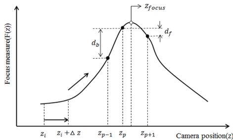
Figure 2: Distribution of focus measure for autofocusing.
