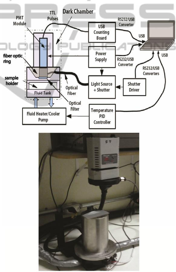
Figure 1: Setup for DL measurements in biosamples - (top) chamber, illumination and controls schematics; (bottom) picture of prototype.
