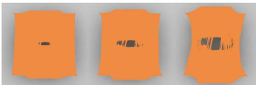
Figure 9: Several successive tears resulting from the propagation of the deformation all along the frailty zone.
