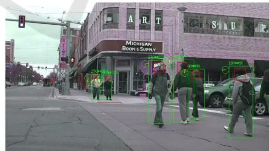
Figure 1: Output of our method. The green boxes are the detected humans. The red boxes are the detected heads. The first numbers are our estimated orientations, and the second numbers are the references.
