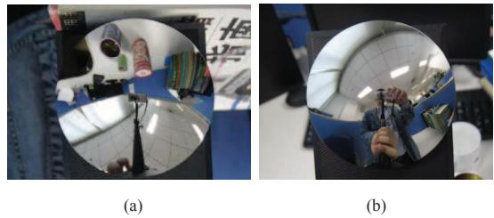
Figure 7: (a) A real image captured by a paracatadioptric camera. (b) The test image.
