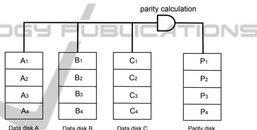
Figure 9: RAID 4 with three data disks and one parity disk.
