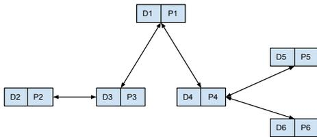
Figure 1: Storage unit partition in sensor nodes.
