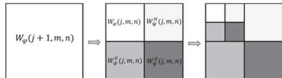
Figure 2: The 2-D Wavelet transform decomposition level  $j$ , along  $m$  rows and  $n$  columns.
