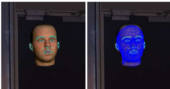
Figure 10: Example of edge and mesh fitting with the particle filter method (zoom on the face area). The inter-eye distance on the input image is 36 pixels.
