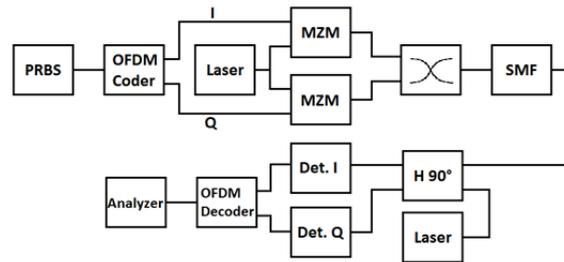
Figure 3: Block scheme of the simulated CO-OFDM system in VPI.
