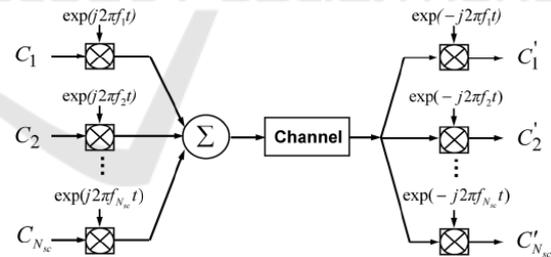
Figure 1: Theoretical implementation of OFDM modulation. (Shieh, 2011).
