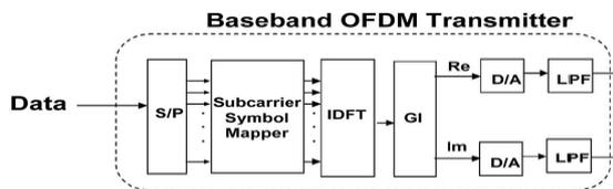
Figure 2: Baseband OFDM transmitter. OFDM modulation is created by IDFT. (Shieh, 2011).
