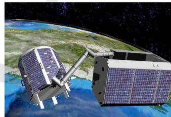
Figure 1: On-Orbit Servicing. Artistic impression of the German on-orbit servicing mission (DEOS); the robot arm mounted on a servicer satellite (right) is grasping the client satellite (left). ©SpaceTech GmbH
