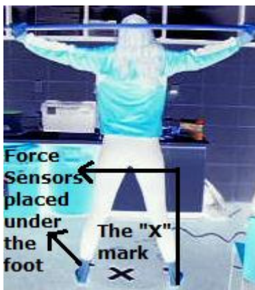
Figure 6: Experimental WBASN set-up for the overhead squat.
