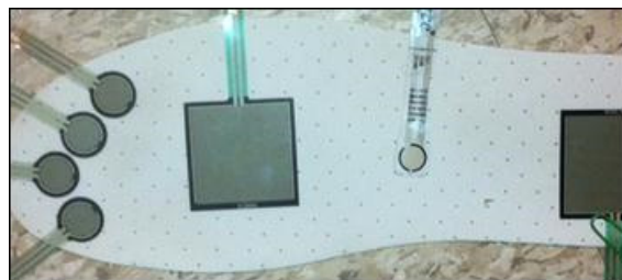
Figure 2: Flexiforce sensors arranged in shoe sole.
