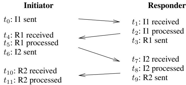
**Fig. 3.** Measured time values  $t_0, t_1, t_2, \dots, t_{11}$  in HIP Base Exchange with IBE signatures.
