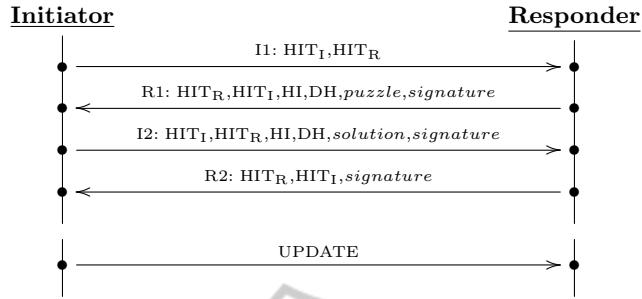
**Fig. 1.** HIP Base Exchange.
