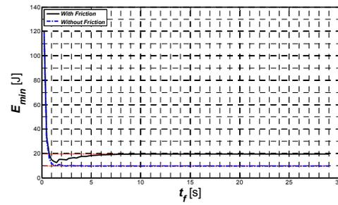
Figure 5: Minimal energy for pendulum lifting with and without friction vs. Lifting Time  $t_f$ .
