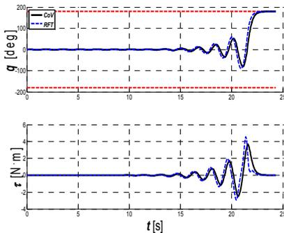
Figure 6: Comparison of  $q(t)$  and  $\tau_{max}$  calculated by using CoV and Reversed Falling Trajectory (RFT).
