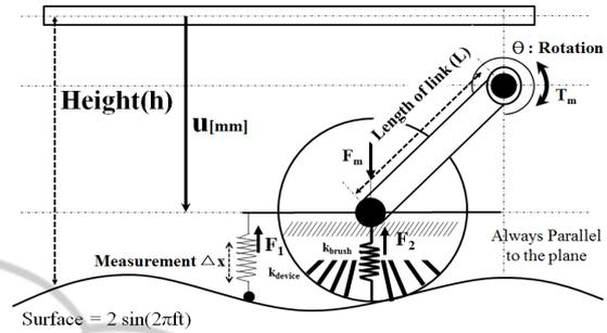
Figure 3: Free Body Diagram of the rotating brush of the robot arm contacting the surface of the duct.
