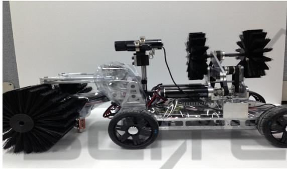
Figure 2: Prototype of Duct Cleaning Robot.
