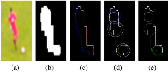
Figure 3: (a) Input image, (b) foreground/background segmentation of the input image, (c) chain code representation of the outer contour: *left*- and *right*-values (yellow and light blue/horizontal lines) of the chain code are of particular interest, (d) detected Hough circles (gray/smaller circles) and circular RoI  $RoI_{bc}$  in which the CCH is calculated (blue/upper, brown/central and yellow/lower circle), (e) detected Hough circles and identified ball (green/lower circle).
