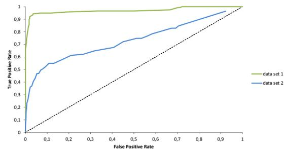
Figure 4: ROC curve of the tested second-stage approach: the ball detection approach for occluded situations. “data set 1” consists of 1408 non-consecutive images: 704 of them showing the ball close to a player or partially occluded by a player and the other 704 images don't show a ball. “data set 2” consists of 9634 consecutive images: 111 of them showing the ball close to a player or partially occluded by a player and 9323 images don't show the ball.
