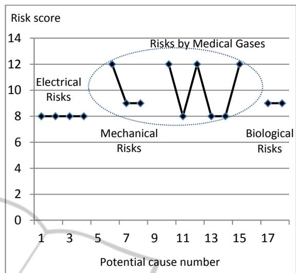
Figure 1: Graphic of the risk scores of the electrical, mechanical, by medical gases and biological risks.
