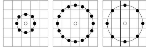
Figure 2: LBP operator examples : circular(8,1),(16,2) and (8,2).
