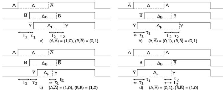
Figure 5: Time diagram of the evaluated signals at the output of a basic DDPL AND/NAND cell for all possible inputs.
