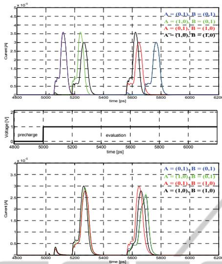
Figure 11: Superimposition of current traces for a basic (upper) and an optimized (lower) AND/NAND gate.
