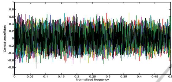
Figure 16: Correlation frequency power analysis on a DDPL S-box without early evaluation (N = 1000).
