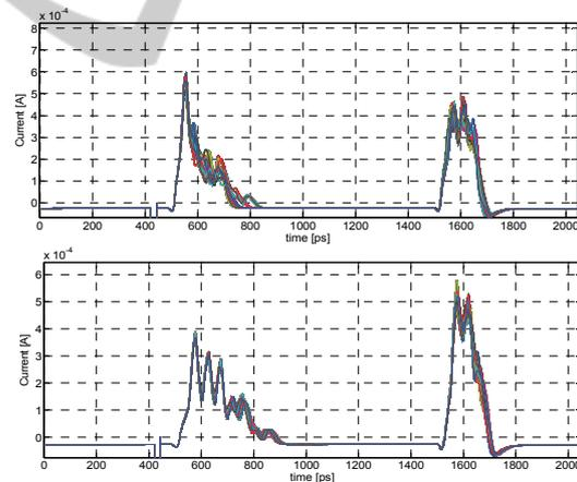
Figure 15: Superimposition of the current traces for the S-Box with (upper) and without (lower) early evaluation.
