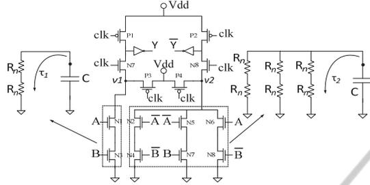
Figure 8: An optimized DDPL NAND/AND gate with the equivalent circuits of the evaluation network.
