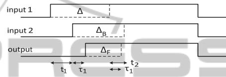
Figure 7: Time diagram of the evaluated signals at the output of a basic DDPL XOR/NXOR cell for each input.
