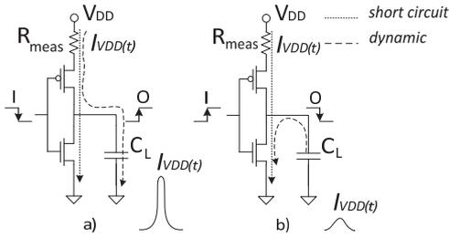
Figure 1: Model of power consumption of an inverter.
