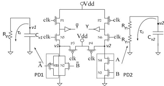
Figure 4: A basic DDPL AND/NAND gate with the equivalent circuits of the evaluation network.
