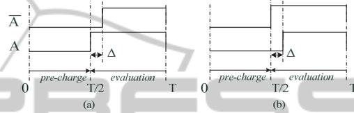
Figure 2: Time domain encoding. (a) Logic-1, (b) Logic-0.
