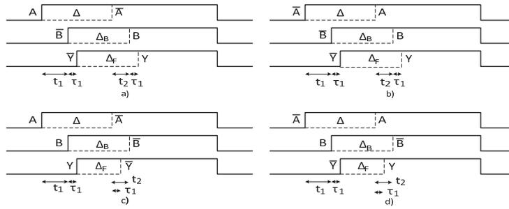
Figure 9: Time diagram of the evaluated signals at the output of an optimized DDPL AND/NAND cell for each input.
