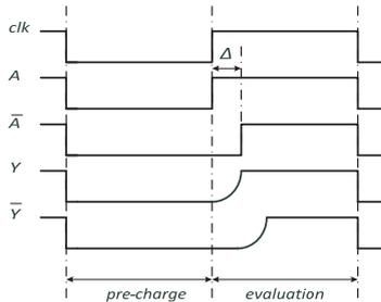
Figure 4: Time diagram of the NOT/BUFFER signals.
