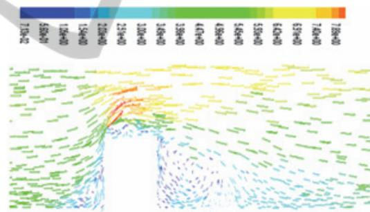
Figure 2: Distribution of longitudinal velocity around buildings.
