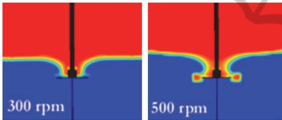
Figure 4: Paddle velocity effect on gas liquid transfer.
