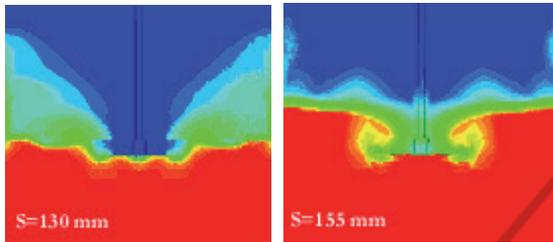
Figure 3: Paddle immersion effect on gas liquid transfer.
