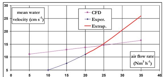
Figure 6: CFD and experimental mean water velocity in the airlift algal pond.
