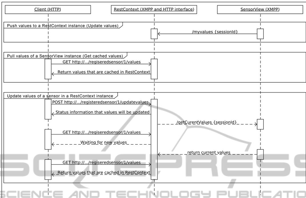
Figure 6: Sequence diagram of communication between a client and a RestContext and SensorView instance.
