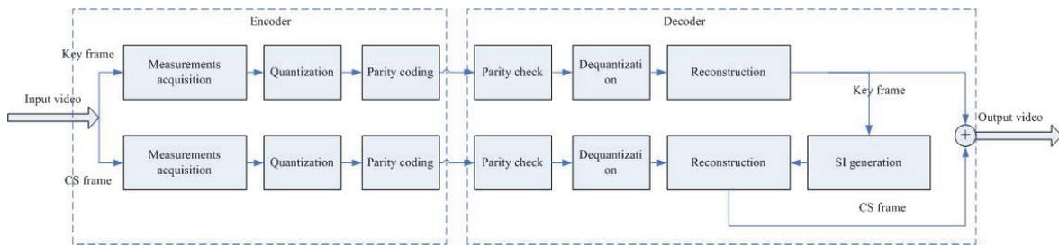
Figure 3: Improved DCVS codec scheme.
