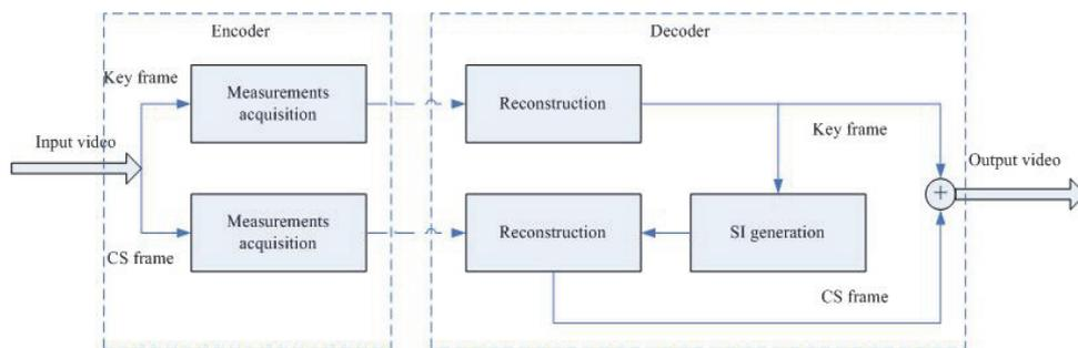
Figure 2: DCVS codec scheme.
