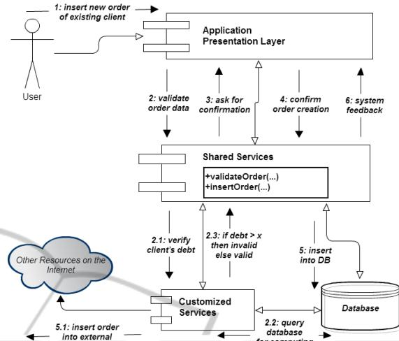
Figure 4: Illustration of an example of the SaaS customizable multi-tenant application.
