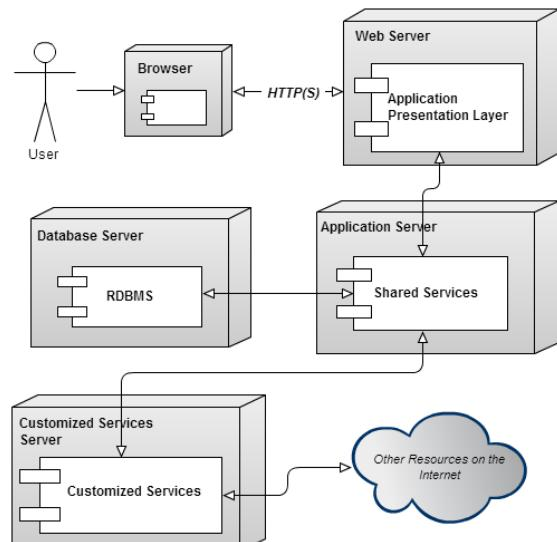
Figure 3: Architecture of the SaaS customizable multi-tenant application.
