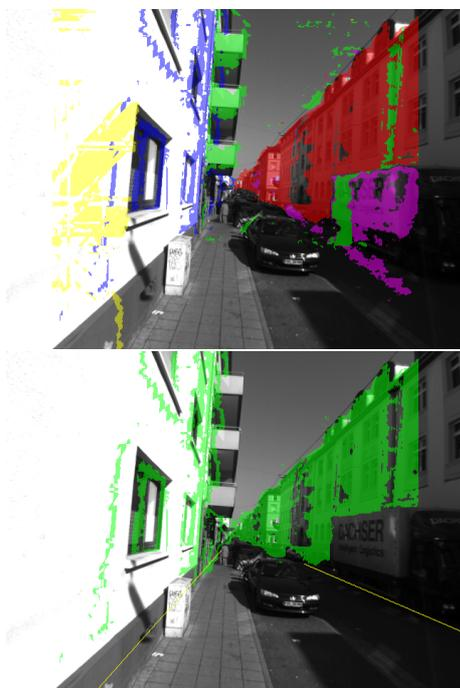
Figure 3: RANSAC based planar segmentation. The two most parallel planes (bottom) are selected from five hypotheses (top).
