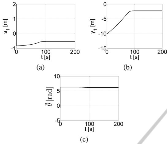
Figure 11: The path following for the unicycle (Soetanto-Lapierre-Pascoal algorithm,  $\theta_a = 2\pi$ ): (a) the distance error  $s_1$ , (b) the distance error  $y_1$ , (c) the orientation error  $\hat{\theta}$ .
