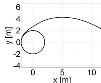
Figure 4: The path following for the unicycle, XY plot (Soetanto-Lapierre-Pascoal algorithm,  $\theta_a = \frac{\pi}{4}$ ).
