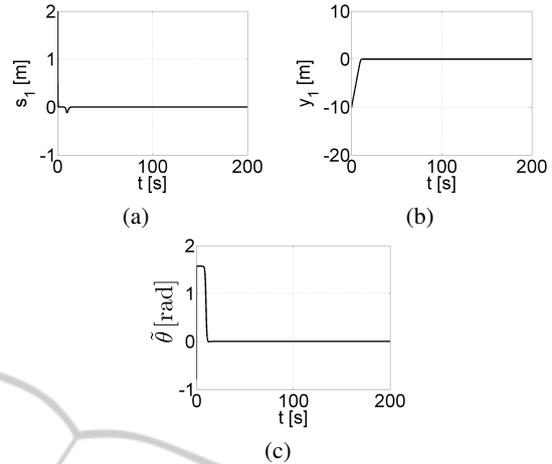
Figure 9: The path following for the unicycle (Soetanto-Lapierre-Pascoal algorithm,  $\theta_a = \frac{\pi}{2}$ ): (a) the distance error  $s_1$ , (b) the distance error  $y_1$ , (c) the orientation error  $\tilde{\theta}$ .
