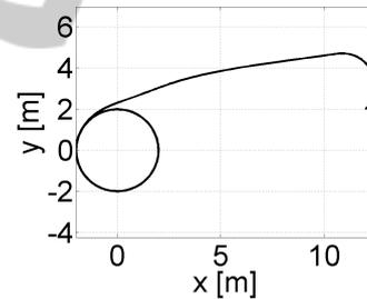
Figure 14: The path following for the unicycle, XY plot (Soetanto-Lapierre-Pascoal algorithm, simulations taking into account velocity constraints).
