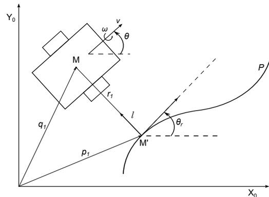
Figure 2: The Serret-Frenet frame definition in a case of an orthogonal projection of a robot on the path.
