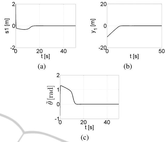
Figure 13: The path following for the unicycle (Soetanto-Lapierre-Pascoal algorithm,  $k_1 = 1, k_2 = 10$ ): (a) the distance error  $s_1$ , (b) the distance error  $y_1$ , (c) the orientation error  $\hat{\theta}$ .
