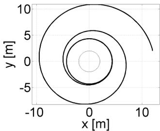
Figure 7: The path following for the unicycle, XY plot (Soetanto-Lapierre-Pascoal algorithm,  $\theta_a = 2\pi$ ).
