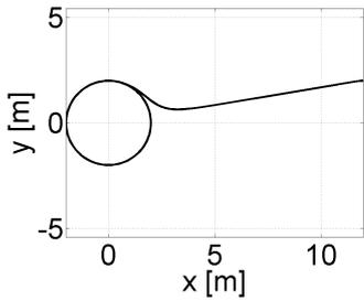
Figure 5: The path following for the unicycle, XY plot (Soetanto-Lapierre-Pascoal algorithm,  $\theta_a = \frac{\pi}{2}$ ).
