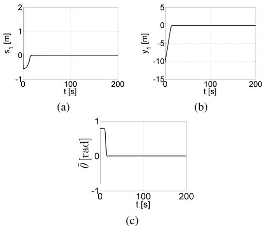
Figure 8: The path following for the unicycle (Soetanto-Lapierre-Pascoal algorithm,  $\theta_a = \frac{\pi}{4}$ ): (a) the distance error  $s_1$ , (b) the distance error  $y_1$ , (c) the orientation error  $\tilde{\theta}$ .
