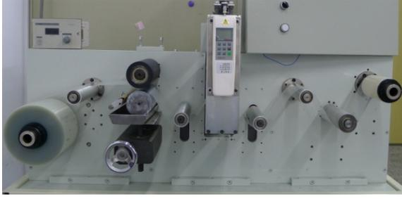
Figure 1: Photograph of the R2R machine.
