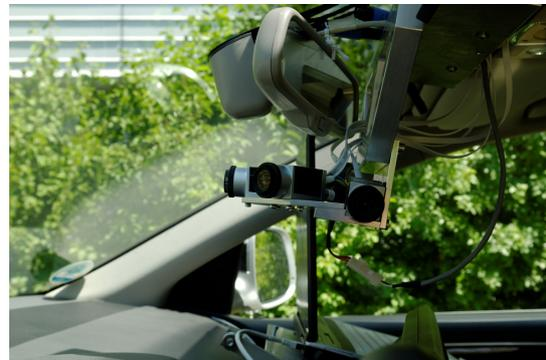
Figure 3: Front camera system covering a field of view of 240 degrees with five cameras.
