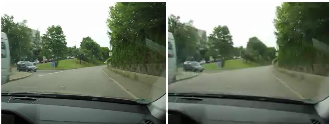
Figure 4: Comparison of video compression with high (640x480, 25.0 crf) and low (320x240, 30.0 crf) quality.
