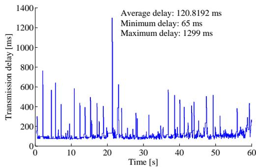
Figure 5: Measured transmission delays during test drives using a 3G network.
