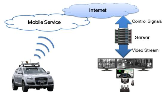
Figure 1: Data transmission scheme for teleoperated road vehicles.
