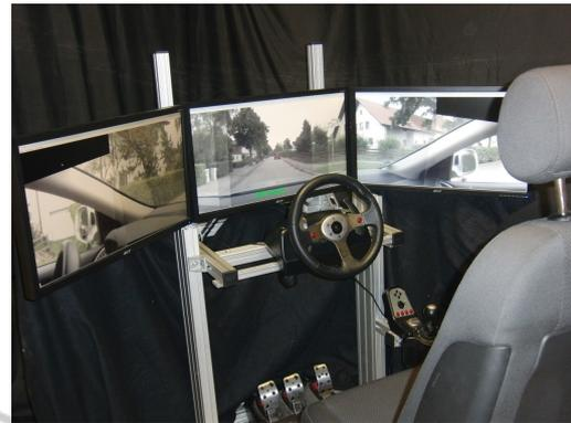
Figure 6: Operator workstation with three monitors, control inputs, and driver seat.
