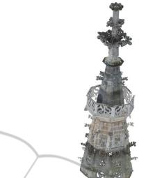
Figure 5: The six point clouds captured from the scaffold registered into a common coordinate system.
