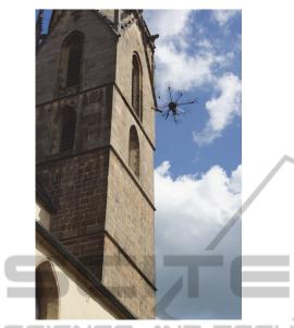
Figure 3: The octocopter collecting images at the southwest side of the tower.
