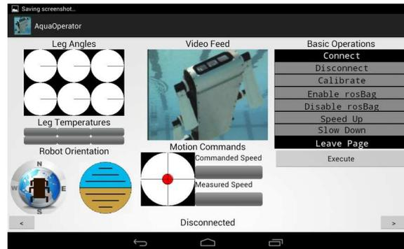
Figure 4: The lightweight AquaTablet user display. The user interacts with the device through tilting the device and also through two two-way switches mounted on the side of the housing. Pitch and roll of the device are used to control the pitch and heading of the robot. See text for details.
