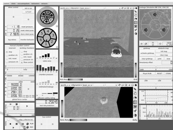
Figure 7: GUI with visualization plugins of the simulated scene (middle), control elements (left), and state information of adhesion (top left) and sealing simulation (top right).
