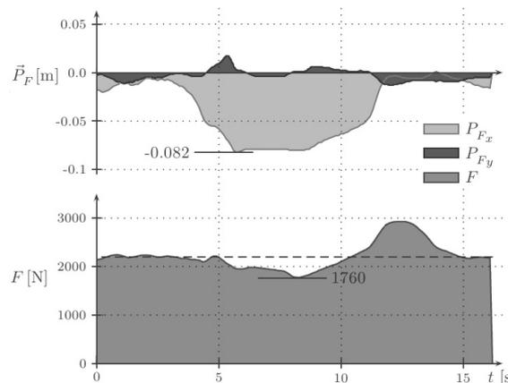
Figure 9: Progress of simulated downforce  $F$  and its point of action  $\vec{P}_F$  during the presented experiments. Robot tilt leads to a shifted point of downforce in vertical direction from seconds 4 to 12.
