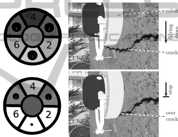
Figure 8: Screenshots of experiment showing the simulated robot CROMSCI driving to a deep crack (right) and current states of the negative pressure chambers (left).
