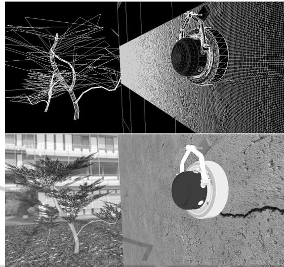
Figure 2: Wireframe model of CROMSCI and a bridge including a band of rough structured surfaces (top) and rendered visualization (bottom).
