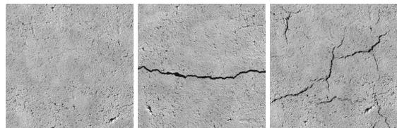
Figure 4: Surface patches with a general roughness, a straight crack and a complex crack structure (from left).
