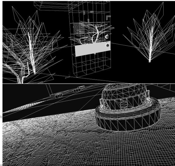
Figure 3: Wireframe model of the environment including the cube elements of the bridge (top) and detailed view of CROMSCI on a rough structure mesh (bottom).
