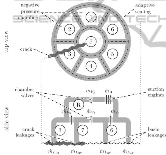
Figure 5: Structural setup of CROMSCI's adhesion components: Adhesion chambers 1 to 7 and reservoir  $R$  with an exemplary crack below chambers 3 and 7.
