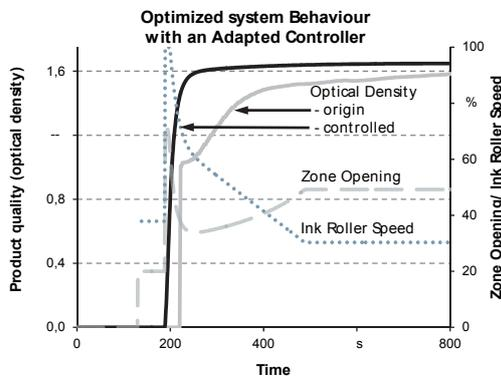
Figure 9: System dynamic with a model based controller.
