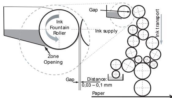
Figure 5: Physical explanation of the offset.
