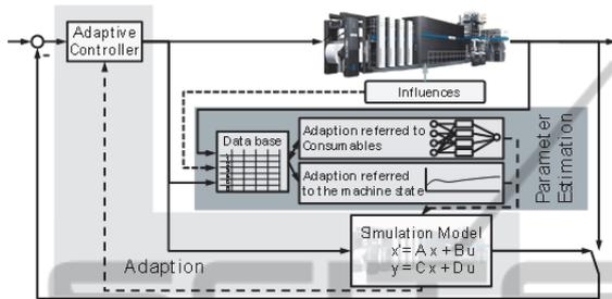
Figure 2: Model based control with parameter adaption.
