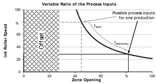
Figure 4: Variable ratio between ink fountain roller speed and zone opening.
