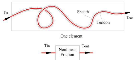
Figure 4: Model of tendon sheath with one element.
