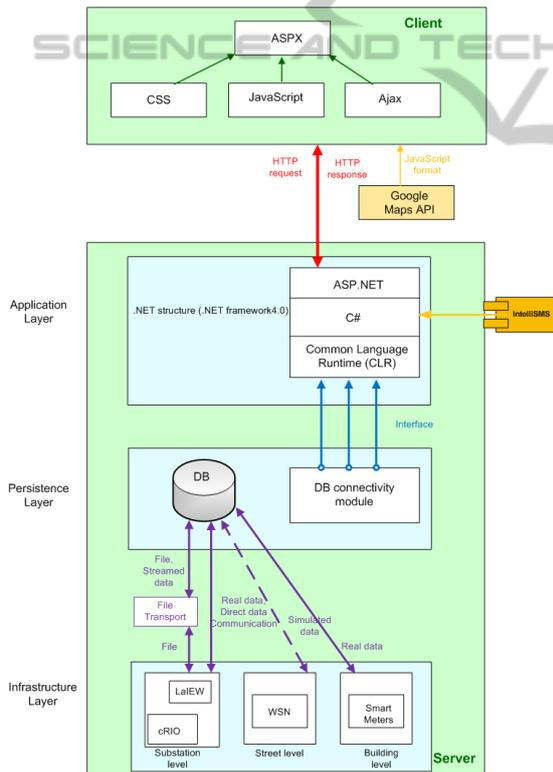
Figure 1: The developed software architecture.
