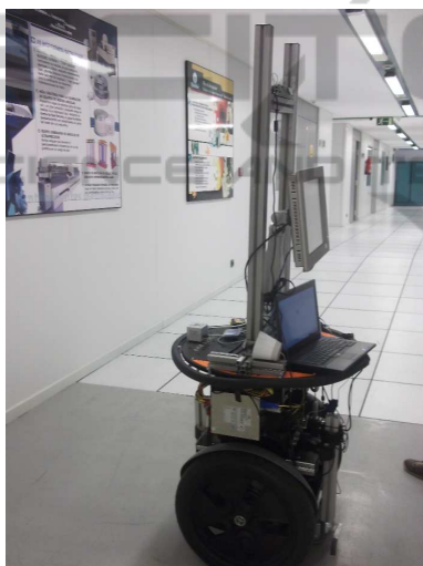
Figure 1: The used robotic platform: a Segway RMP 200 provided with the Kinect and the thermal sensor.
