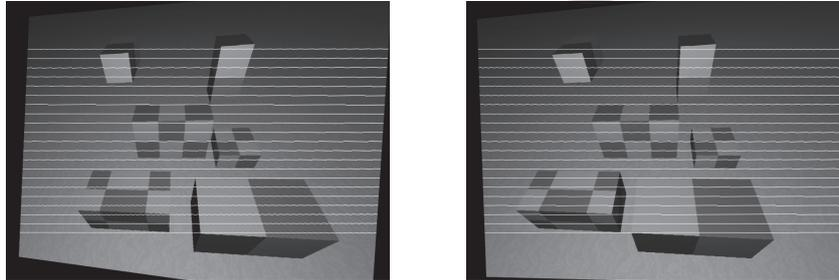
**Fig. 5.** Stereo pair rectified from the estimated fundamental matrix.
