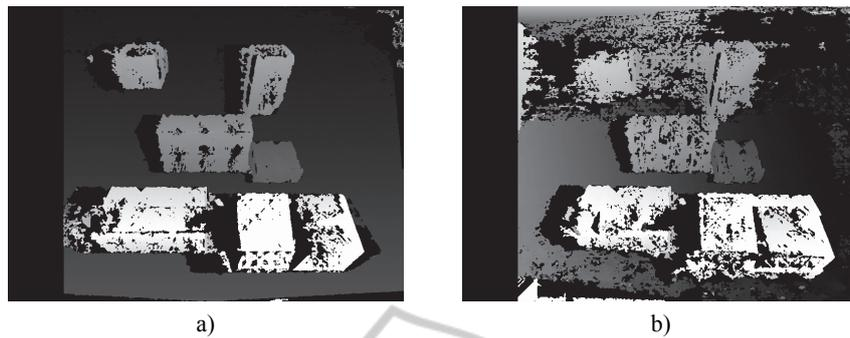
**Fig. 6.** Disparity map for: a) exact fundamental matrix, b) estimated fundamental matrix.
