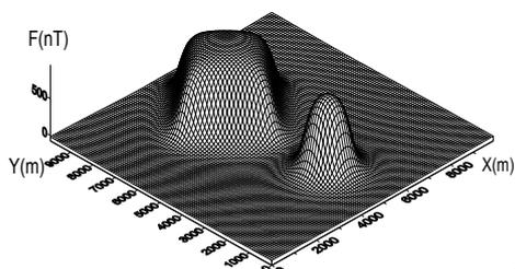
Figure 1: Magnetic anomaly map of the synthetic model.
