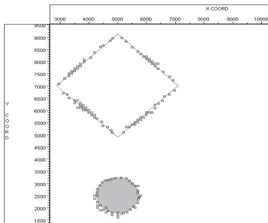
Figure 3: Structural boundaries delimited by the 2D CWT.
