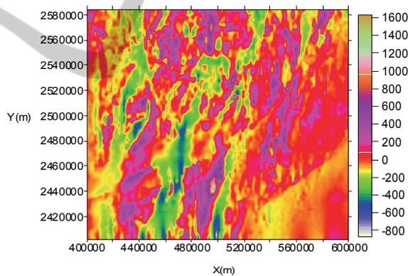
Figure 5: Magnetic anomaly map reduced to the pole.
