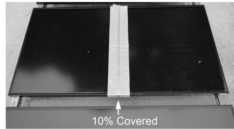
Figure 9: PV module #19 with covering of 10% total area.
