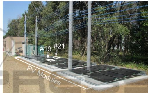
Figure 1: Photograph of the monitoring system for individual PV modules (with modules #19 and #21, used in this paper, highlighted).
