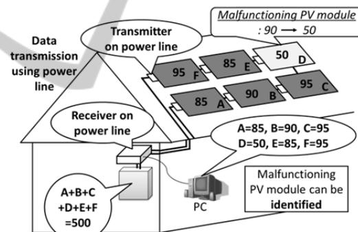
Figure 2: Overview of the monitoring system for individual PV modules.
