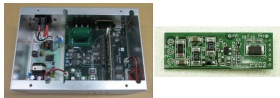
Figure 3: Transmitter (left, 197 x 140 x 75 mm) and receiver (right, 14.5 x 42.0 mm) for the PV module monitoring system.
