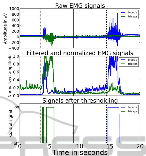
Figure 6: Resulting signals after preprocessing and thresholding: (top) Raw EMG signals from biceps (blue) and triceps (green), (middle) filtered and normalized signals, and (bottom) results of the thresholding algorithm.
