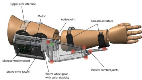
Figure 2: Mechanical design of the active Orthosis. The red dots represent the positions of the passive degrees of freedom.
