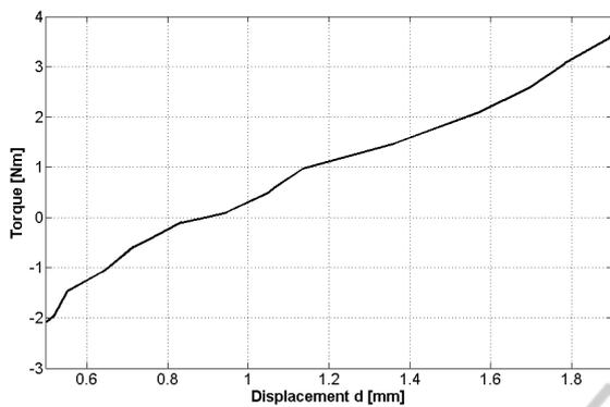
Figure 4: The calculated joint torque - deflection curve.
