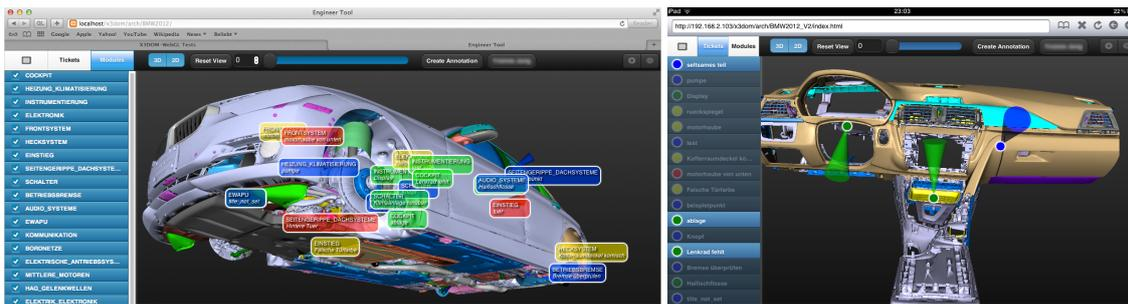
Figure 1: A 91M triangles CAD model of a car consisting of several base modules with 2D and 3D annotation markers, rendered in a common Web Browser at real-time frame rates. Left: Using a desktop PC. Right: Using an iPad 2.
