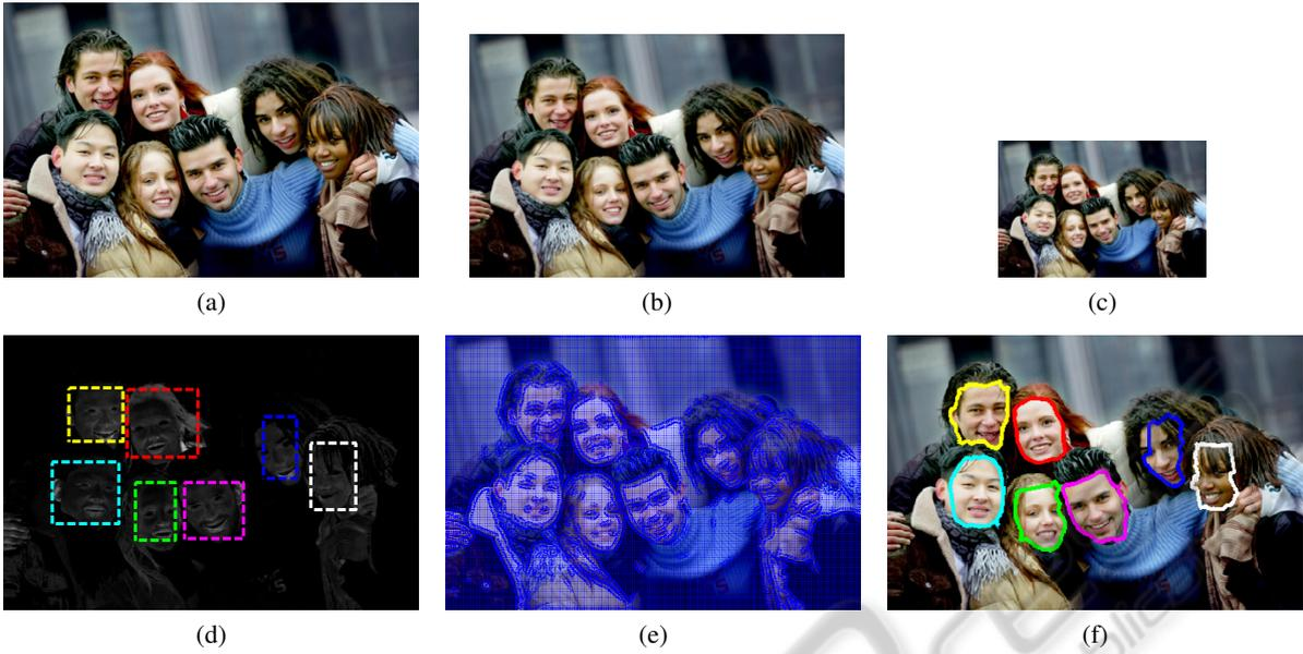
Figure 3: Our system's performance in the case of multiple face detection in an image of a group consisting of several persons with diverse gender and origins: (a) original image; (b)-(c) downsampled images; (d) initial active contours; (e) multi-scale, multi-feature vector flow field; (f) final active contour results.
