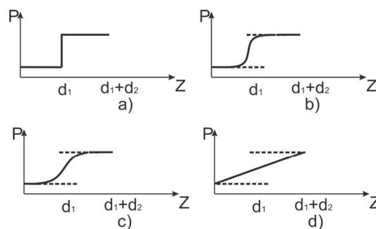
Figure 1: The model of ChLC pitch's profile: a) at the beginning of diffusion, b),c) in the middle of diffusion process and d) at the end of diffusion.
