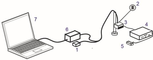
Figure 2: Scheme of experimental set-up for investigation of discussed system's reflection and transmission spectra: 1. Tungsten-krypton lamp, 2. CLC cell, 3. Microrefrigerator, 4. Controller of temperature, 5. Tester, 6. Spectrometer, 7. PC.
