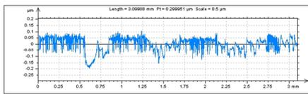
Figure 3: Typical surface roughness scan using the Talysurf PGI 1000 made on one of the polished ends of the sample.
