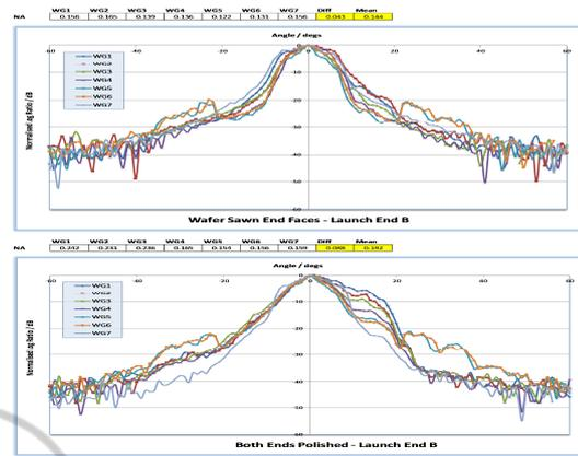
Figure 8: Far-field intensity scans of waveguide group containing 7 individual waveguides. Graph shows normalised signal against angle on sample with wafer sawn and polished end faces with a launch at End B. Also shown are the calculated numerical apertures of each waveguide.
