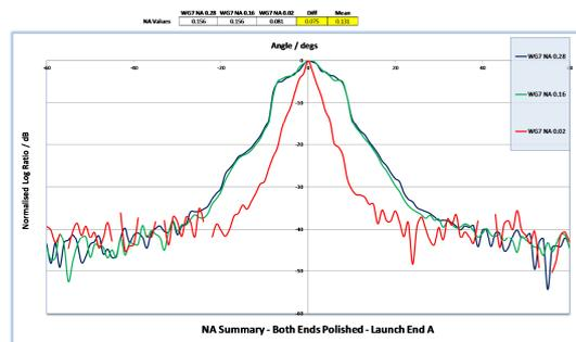
Figure 6: Far-field intensity scans of selected waveguides. The graph shows normalised signal against angle on sample with optically polished end faces with a launch at End A. Also shown are the calculated numerical apertures of each waveguide.
