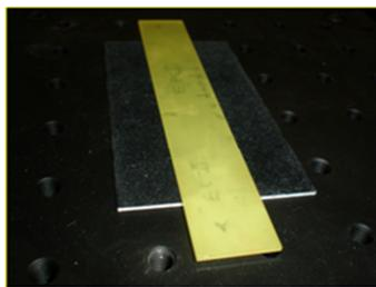
Figure 4: Sample OPCB containing groups of planar siloxane waveguides.
