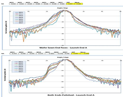
Figure 7: Far-field intensity scans of waveguide group containing 7 individual waveguides. Graph shows normalised signal against angle on sample with wafer sawn and polished end faces with a launch at End A. Also shown are the calculated numerical apertures of each waveguide.
