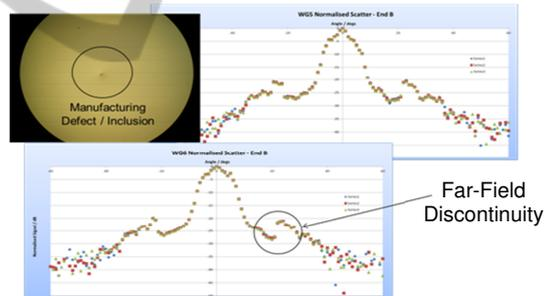
Figure 9: Far-field intensity scans of selected waveguides 5 and 6 affected by identifiable defect along waveguide length.
