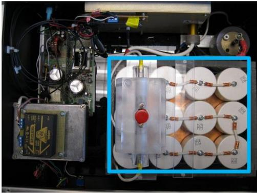
Figure 1: Picture of internal architecture of the nanosecond pulse electric field generator; the pulse forming network is highlighted in blue.
