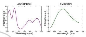
Figure 2: Absorption and emission spectra of flavins.
