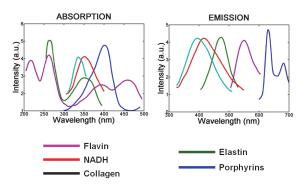
Figure 5: Absorption and emission spectra of some proteins.
