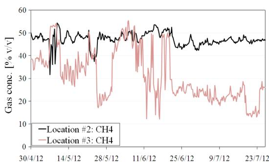
Figure 7: Methane readings from locations #2 and #3.
