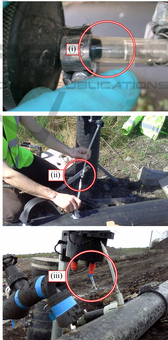
Figure 4: Site-specific issue rectification (i) Waterblockage, (ii) Tube shrinkage, (iii) Connection breakage due to pipe collapse.
