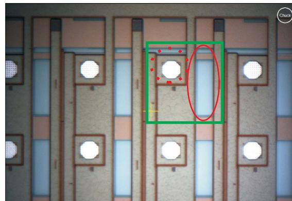
Figure 3: Photo of a single pixel. The vertical and horizontal pitch is 70 $\mu\text{m}$ .
