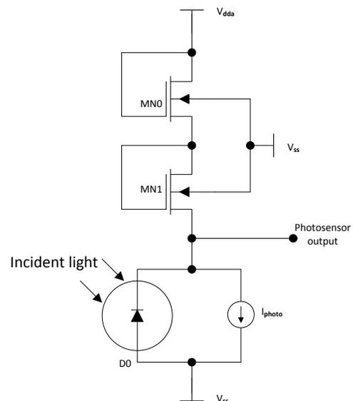
Figure 1: The photosensor circuit fabricated and investigated in this study.
