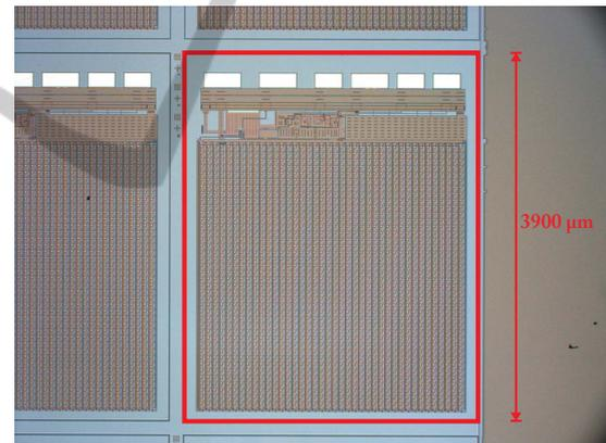
Figure 2: The chip micrograph: A single chip is inside the red rectangle.
