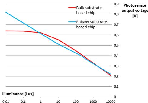
Figure 4: The characteristics of the photosensor output voltage versus illuminance for bulk and epitaxy substrate based chips.
