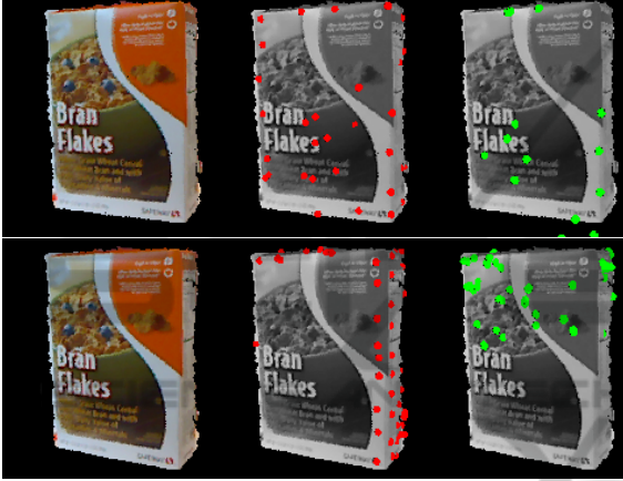
Figure 2: Hybrid keypoints on cereal boxes from the RGB-D dataset. 3D keypoints are displayed with red spheres, hybrid keypoints are displayed with green spheres. Notice that the red spheres location is different from the green ones due to the added intensity variation. First row corresponds to Harris detectors and second row to SUSAN detectors.
