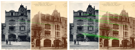
Figure 9: Valid matches obtained with the homography ground truth estimate, using the SIFT detector-descriptor (left) and the ASIFT algorithm (right).
