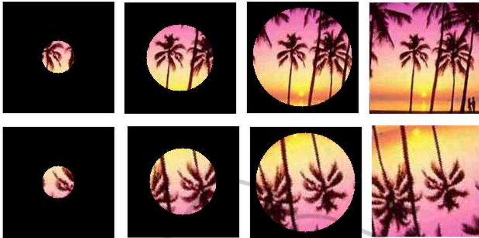
Figure 2: This figure shows the same images of Figure 1. The original image of the BACKGROUND_Google class of Caltech-101 database and the image rotated in 196^\circ . It shows the 4 regions of the PCCR approach for each image. The first column shows the first circular region with radius of 15% of image's height, the next column shows the second region and so on, until the last column showing the entire image that is the fourth region used to calculate the final descriptor.
