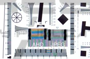
Figure 1: ISO 12233 chart image. Enlarged details are for AHD and in-camera JPEG.
